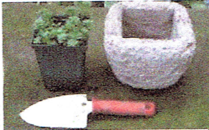
Used the plastic container as mold and applied mixture to outside.
